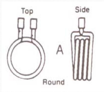
The pancake coil shown below is used for heating flat surfaces.
