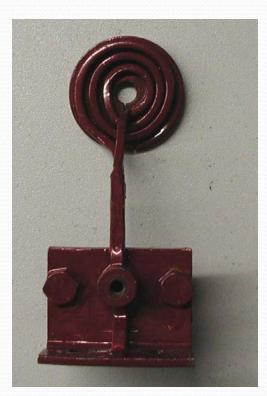
The induction coil quickly raises the temperature of a work piece by means of a high frequency current which passes through the coil, as shown in Fig. 1.
