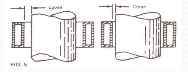
When multi-turn coils are closely coupled to a workpiece, there is a tendency for the eddy-currents to create a heat pattern matching the coil's helix.
