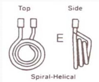
The spiral-helical coil shown above is used for heating conical surfaces.
